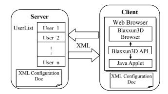
Figure 2. Proposed new VNet system architecture for extensible animations
