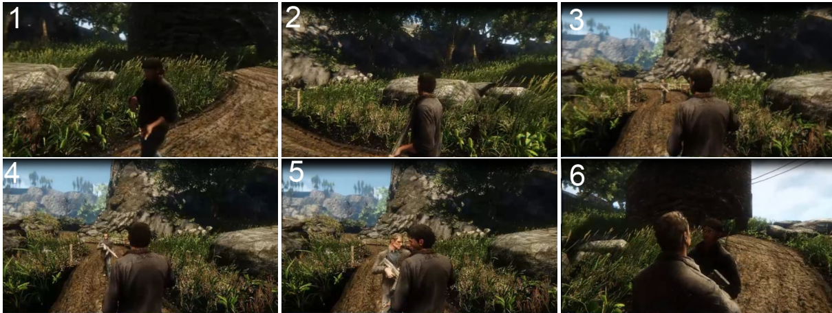
Figure 11: Resulting shots from trajectories generated by our camera motion graph process, making a transition between a one target trajectory and a two target trajectory (between shots 2 and 3).
