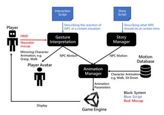
Fig. 1. System architecture.
