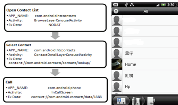
Figure 9. Left: Steps for placing a call through contact list Right: Screen for contact list
