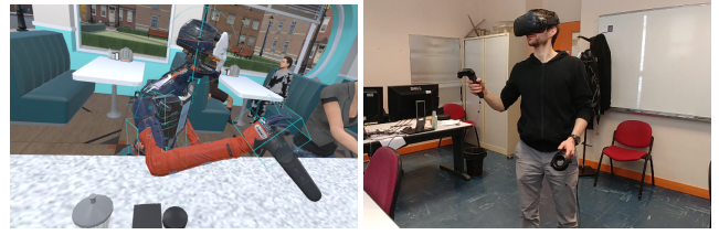
Figure 5: We propose a novel interacting metaphor to craft character poses with Inverse Kinematics to ensure the naturalness of the pose. Starting from an initial pose (Left), the user can create new poses through a small set of operations.
