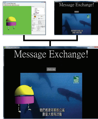
Fig. 1. Integration of external 3D animation system to overlay a virtual character on TV.
