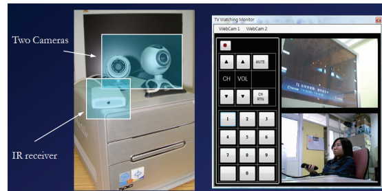
Fig. 3. Setup and Snapshot of event recording tools.
